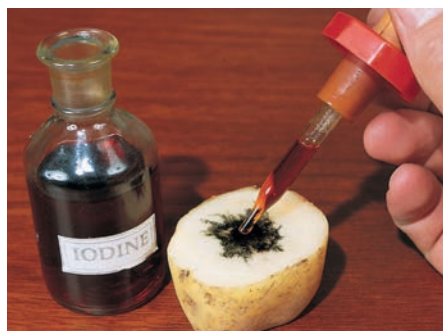
Figure 2.1 When iodine–potassium iodide solution encounters starch, its colour changes from orange–brown to blue–black.
