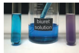
Figure 2.5 The biuret test for proteins. Biuret solution is pale blue but turns pale purple in the presence of protein.
